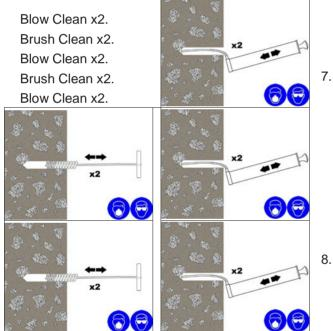
If the hole collects water, the current best practice is to remove standing water before cleaning the hole and injecting the resin. Ideally, the resin should be injected into a properly cleaned, dry hole. However, this product may also be used in a flooded hole.
