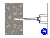
nozzle from the hole ensuring that there are no air voids as the mixer nozzle is withdrawn. Fill the hole to approximately  $\frac{1}{2}$  to  $\frac{3}{4}$  full and withdraw the nozzle completely.
